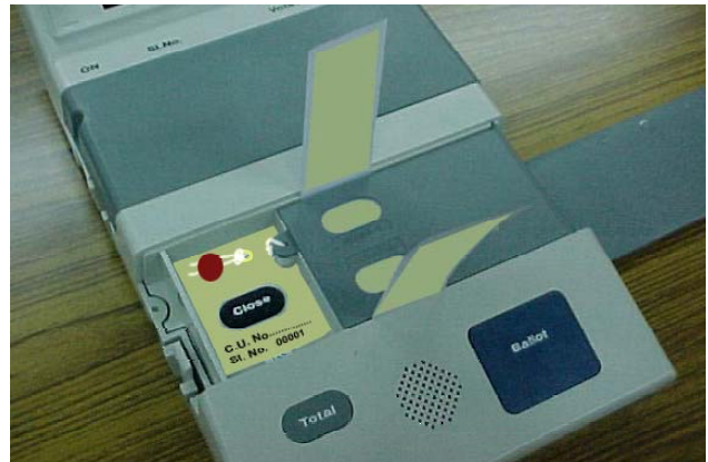
Sealing the inner door with Special Tag ECIL Machine
