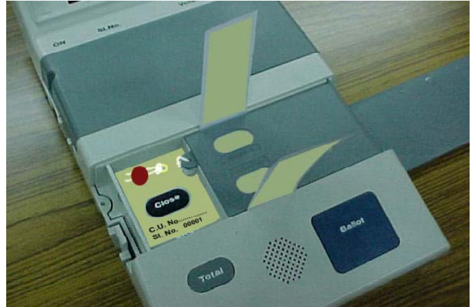
Sealing the inner door with Special Tag
