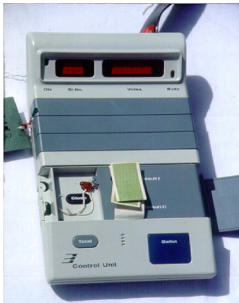
Closing the inner door with thread ECIL Machine
